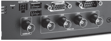
1 x AUDIO-IN + 4 x VIDEO-IN BNC connector for DVR surveillance system
